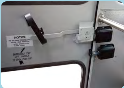
Vandalock - rear door vandal and interlock system
